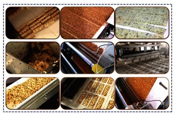
**Detailed Main Equipment Picture Of Candy Fruit Energy Granola Bar Line** Breakfast peanut chikki candy fruit energy granola bar making machine adopts PLC operating system and advanced mechanical structure to realize fully automated Production. The chocolate granola bar making line continuous feeding, automatic flattening, automatic cutting and cross-cutting. Compared with traditional hand-made methods, the cereal bar machine reduces a lot of production costs and improves production efficiency.
